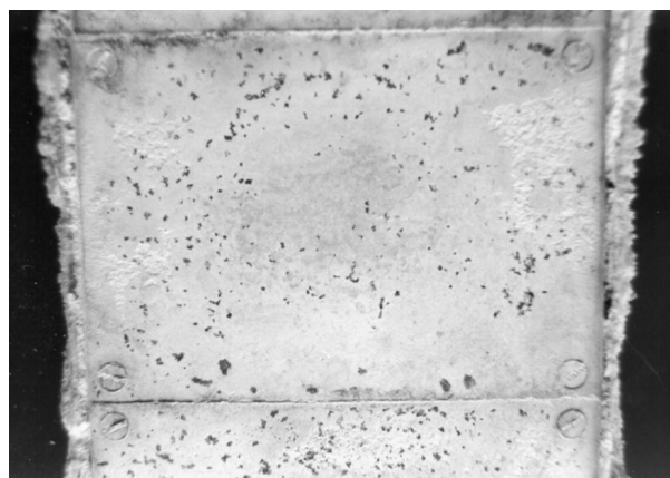
Figure 11. Adhesive side of a fouling layer.
